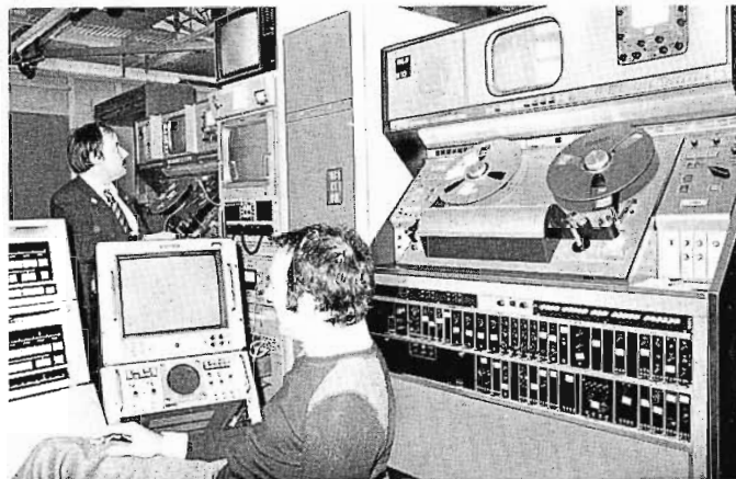
ORF utilized twelve TR-70C's in producing the world program. Four were located in two OB vans. The rest were assigned to four editing suites in which action highlights from many hours of recorded material were quickly assembled. The two machines shown here operated at half speed and were equipped with dual-cue programmer editing systems.
